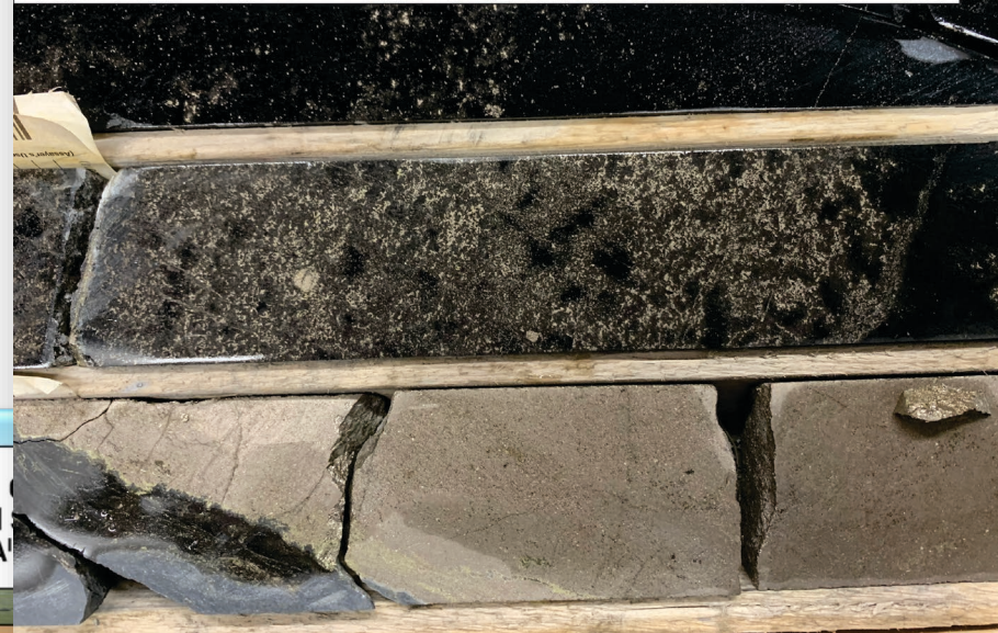
Photo 2: Type 1 Nickel Sulphide Mineralization Hole FAB-18-56 Down hole gradation from disseminated pyrrhotite (Po), pentlandite (Pn) and lesser chalcopyrite (Cp), through net-textured (matrix) to massive sulphides (Po>>Pn>Cp) at base of intersected interval. Interval graded 1.35% nickel over 3.94 metres, including 3.59% nickel over 1.03 metres from massive sulphide
